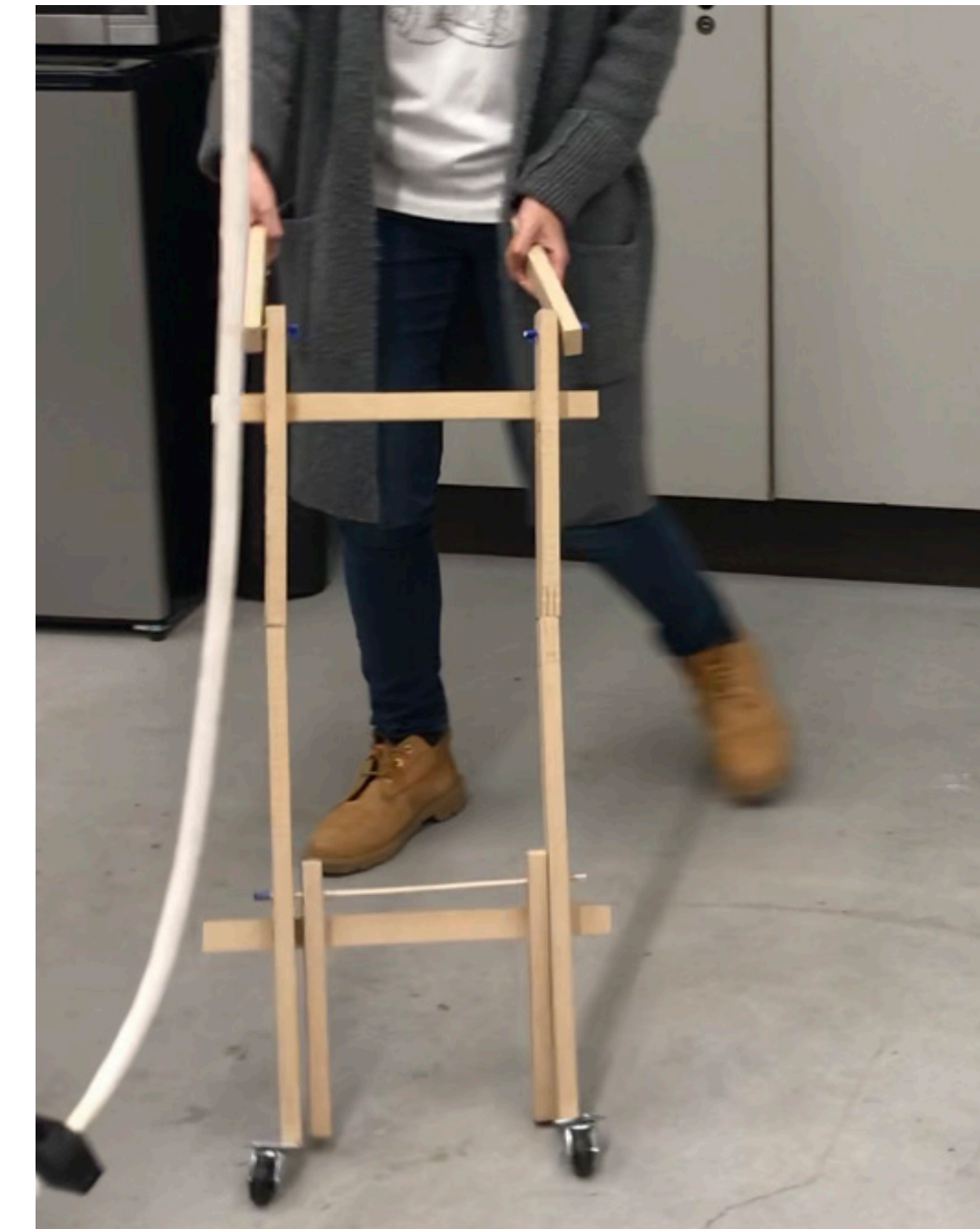
Two wheel system, Hard to control the direction
