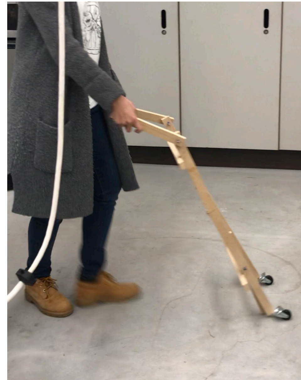
Two wheel system, Hard to control the direction
